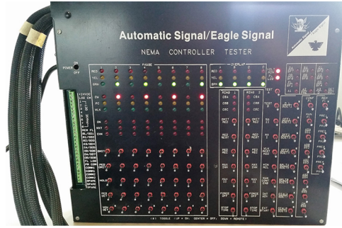
Fig. 6. All-direction green lights being displayed on traffic signal test equipment. The left 4 green LEDs represent the through directions of travel at an intersection while the right 4 green LEDs represent the corresponding left-turn lanes. (Color figure online)
