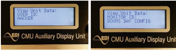
Fig. 5. CMU-212 display unit showing the Datakey configuration for USER ID and MONITOR ID which was written using the home-made Arduino Datakey writer to allow for full-permissive configuration.
